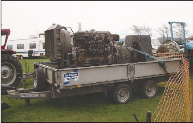
6 LX powered Genset
